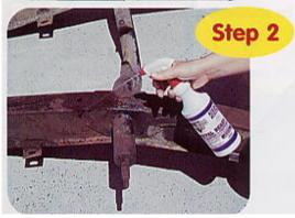
Prepare the rusty or corroded surface with Metal Ready. As a rust remover / preprimer; Metal Ready will neutralise rust, etch metal for better adhesion, and coat the metal with zinc phosphate to encourage deep chemical bonding of POR 15<sup>®</sup> Rust Preventive Paint to the base metal and rust. Leave for 10 minutes. Rinse well with water.
